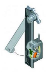
The server cabinets are fitted with electrically opened swing handles including solenoid and mechanically operated latches. Operation may also be arranged via keypad, proximity card, mobile telephone or network-management-stations. Control and sensor modules allow a controlled access and ensure the monitoring or logging of all events.
