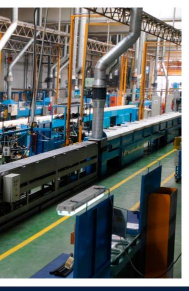
In the further processing department fixed lengths, vulcanised rings and frames can be made to size. Some EMKA branches have machines for vulcanising corner joints. The application of adhesive tape or lubricant varnish completes the range.
