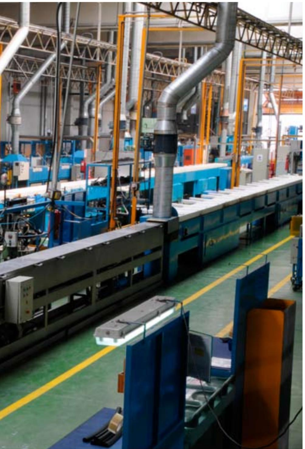
In the further processing department fixed lengths, vulcanised rings and frames can be made to size. Some EMKA branches have machines for vulcanising corner joints. The application of adhesive tape or lubricant varnish completes the range.
